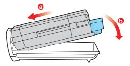
**11.** Push the colored release lever (1) away from you to lock the toner cartridge onto the new image drum unit and release toner into it.
